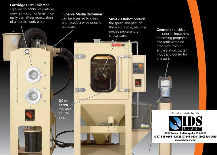
Empire's new RBT36-F robotic pressure-blast system opens the door for many firms to cash in on the benefits of high precision air blasting. Capable of processing parts up to 12 inches in diameter by 12 inches tall, the RBT36-F employs a Fanuc 6-axis robot to control nozzle movement plus a DC or Servo drive to control part movement, enabling users to assure the quality control and deliver the process validation so often required by today's aerospace, automotive and medical-equipment sectors.
